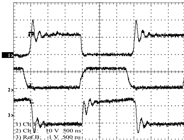
Fig. 15. Full load condition, from top to bottom: voltage across switch 1, gate control signal, current through switch 1 (1V ~ 25A)
